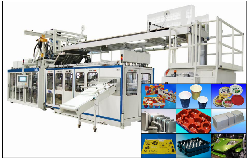
ILLIG RDM 75K air pressure forming machine for manufacture of food cups • Output 100,000 cups per hour in polystyrene • 40 cycles per minute with a cup diameter of 3 inches (75mm)
