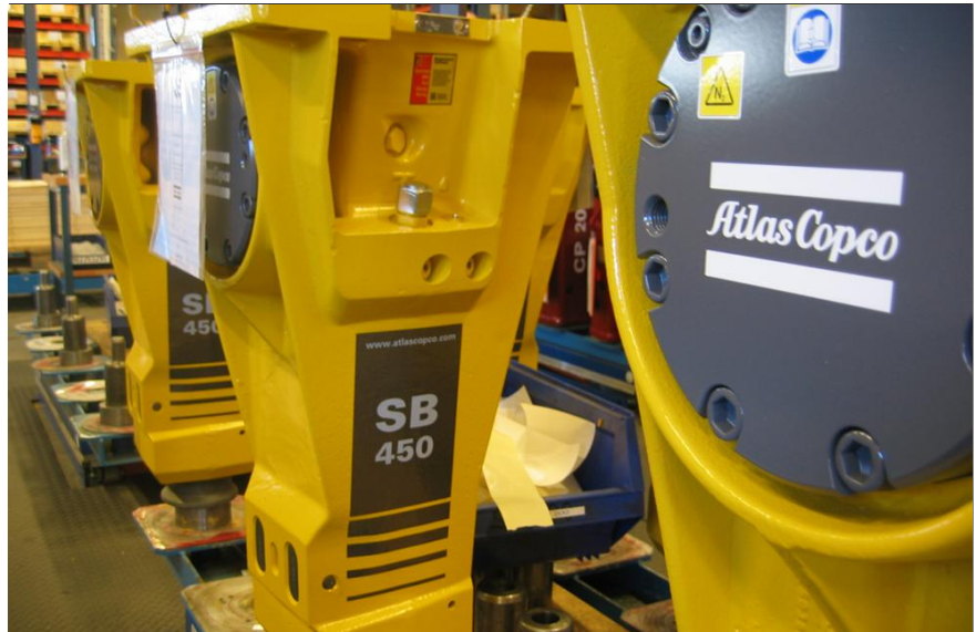
Hydraulic breaker from Atlas Copco in Kalmar, SB 450 Scaler
